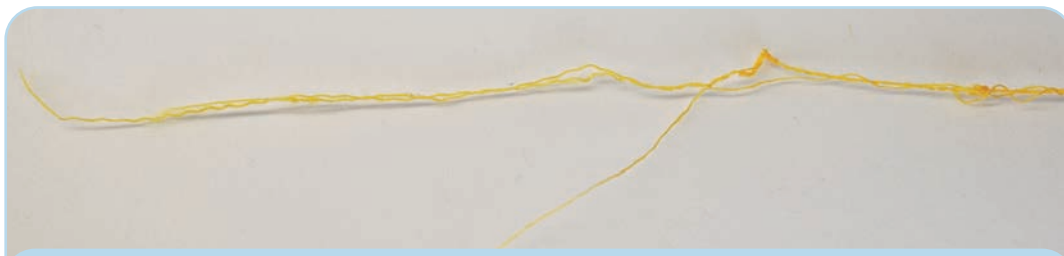
Long Frayed Break: a burr along the thread path snagged and ripped the thread.
