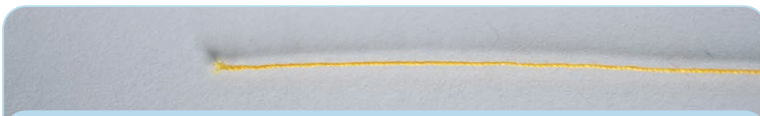
Clean Break: often caused by poor needle orientation or a bent needle.
